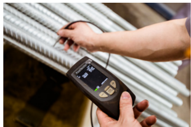
Control of coating thickness
